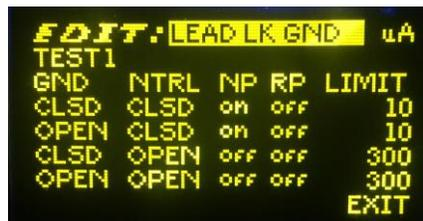
5. Press **START** to advance to **EDIT: LEAD LK ISO** tests. Use UP/DOWN arrow keys to highlight value to be edited. Press **START** to edit value. When Limit value is flashing, use UP/DOWN arrow keys to change value. Press start again to accept edited value.
