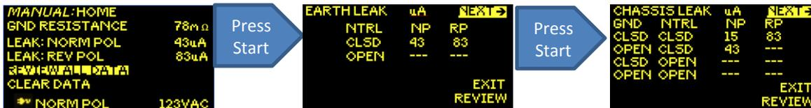
**NOTE:** Tests can be repeated from SUMMARY screens. Highlight test using up down arrow keys, press **START** to begin. Press **START** again to end test.
