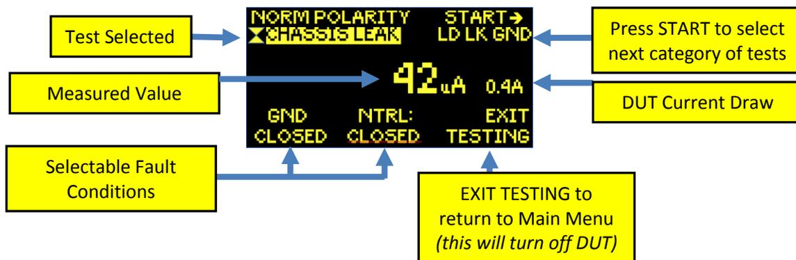
4. Use **UP** or **DOWN** arrow keys to change fault conditions e.g. GND CLOSED to GND OPEN and NTRL CLOSED to NTRL OPEN.
