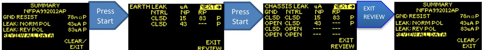
5. **Retesting in Auto Review Screens:** From REVIEW screens for any test completed, the result can be reviewed and repeated by scrolling to that line using up or down arrow keys and pressing **START** key. The test will repeat and the new test result will replace the prior. This can be done for any test turned on in the Auto Profile, but not for any test that was turned off in that profile.
