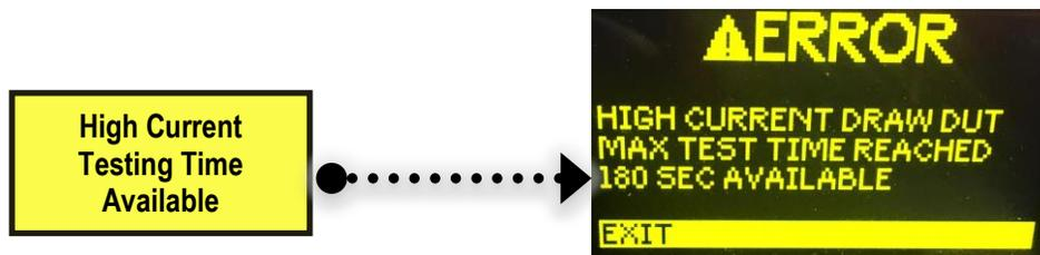
\*Safe-T Sim is designed to continuously track the amount of time that high current is being drawn by the DUT in order to ensure to limit the time to a maximum of 180 seconds.
