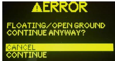
**NOTE:** If you are using the ST-1 in an isolated power environment that is causing this message and are confident it will not affect accuracy of electrical safety measurements, select **CONTINUE** to begin testing.
